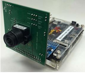
Fig. 6. A hardware system prototype with an SK-Hynix mobile image sensor.
