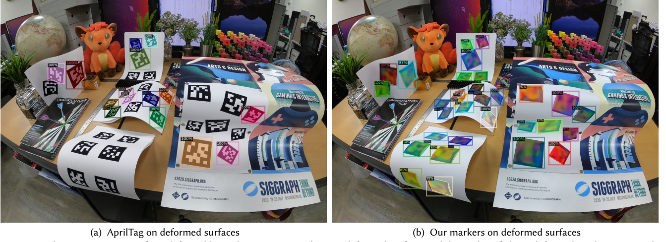
Fig. 18. Qualitative comparison of our deformable markers against AprilTag on deformed surfaces. While AprilTag fails on deformed markers, our method detects all the markers on deformed surfaces.
