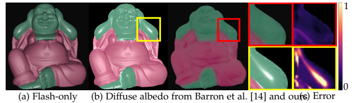
Fig. 2: Modeling specular appearance is essential. Diffuse albedo recovered from Barron et al. [14] (b left) using flash-only image (a) and depth as input. Our approach with specular modeling given added no-flash input (b right). Since Barron et al. compute diffuse reflectance only, specular highlights cannot be factored from diffuse albedo. (c) shows difference from ground truth.
