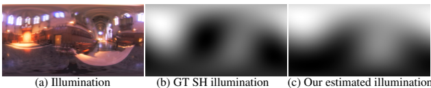
Figure 7: (a) Illumination (a.k.a. Grace) used for creating a synthetic dataset, shown in Figure 8. (b) GT illumination projected to 2nd-order spherical harmonics. (c) Our estimated illumination. Our method successfully estimates low-frequency illumination.
