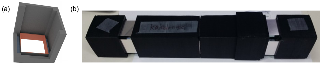
Figure 5.3: Building the kaleidoscope. (a) presents a 3D model of our kaleidoscope holder, and (b) shows constructed kaleidoscope using four first-surface mirrors with two holders.
