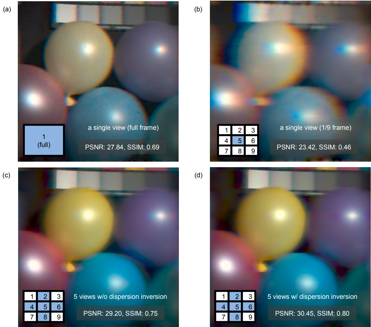
Figure 6.2: (a) The traditional CASSI system [45] synthesized with a full-frame input ( 1935 \times 1503 ), which has a nine times larger resolution than that of a view ( 645 \times 501 ) in our multiview configuration. (b) a reconstruction result using a single view of the multiview configuration. (c) and (d) compare spectral reconstruction results using five different views that we use with our prototype. (c) shows a reconstruction result without dispersion inversion (see Figure 5.1b), while (d) presents a reconstruction results with dispersion inversion. The five-view reconstruction with dispersion inversion improves not only PSNR but also SSIM of spectral channels.
