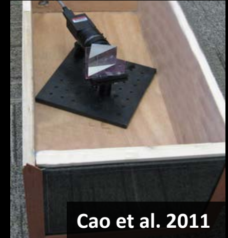
Prism-Mask Multispectral Video Imaging System (PMVIS)
