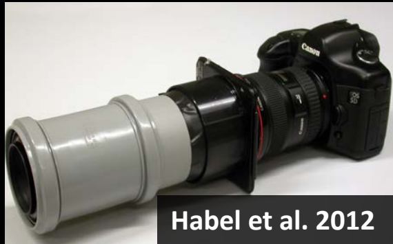
Computed Tomography Imaging Spectroscopy (CTIS)
