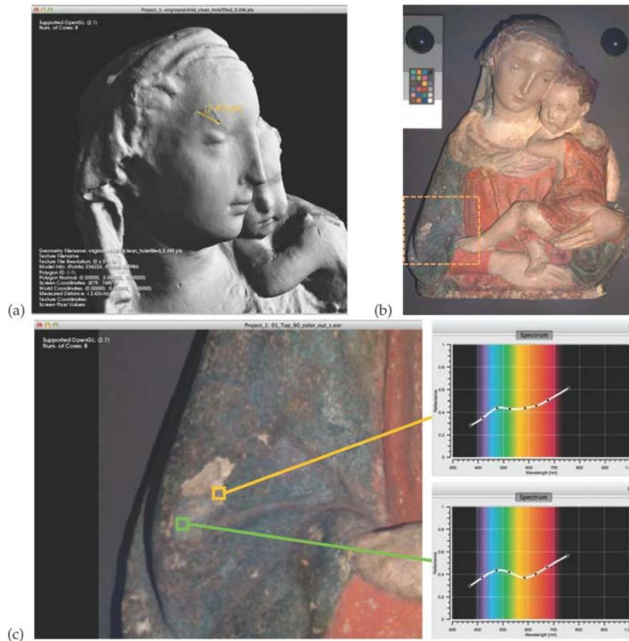
Fig. 7. Polychrome stucco relief, *Virgin and Child*, Italy 15th century, by Vittorio Ghiberti. (a) Measuring the length of the plaster crack in the relief. (b) A hyperspectral image of the object. The rectangle with dotted lines indicates the region shown close-up in the next image. (c) Reflectance spectra of pigments on the hyperspectral image (b) are depicted on the spectral plot widget. The two plots represent data from two different points of interest (the green and yellow squares).
