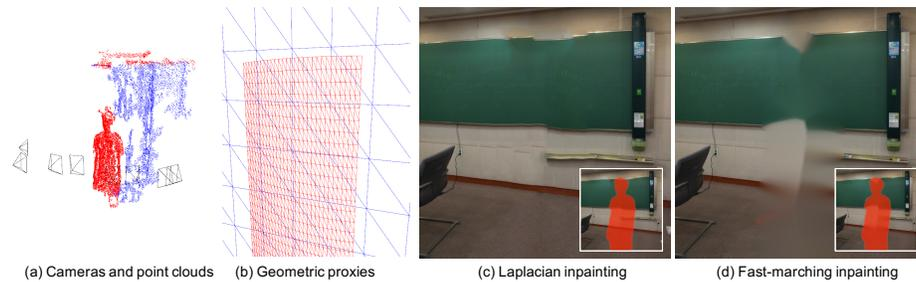
**Fig. 3.** An example of estimated point clouds (a) and proxy geometry (b) of a scene. (c) is inpainted by a Laplacian-based method [8] in 362 secs. (d) is completed by a fast-marching method [19] that we chose in 1.07 secs. Insets show inpainted regions.
