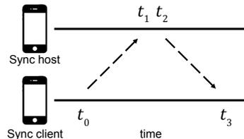
Fig. 2. Packet-based synchronization.
