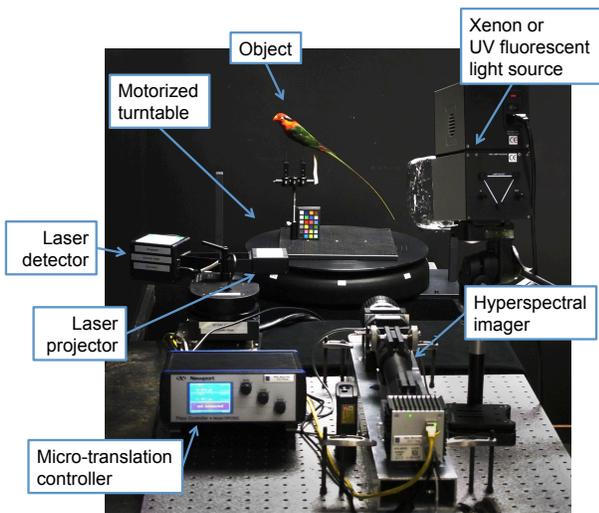
**Fig. 2:** Overview of the 3D imaging spectroscopy system [17]. The system includes a custom-built hyperspectral imager, a laser scanner, a turntable, and xenon/ultraviolet light sources.
