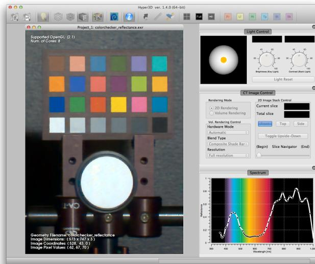
**Fig. 5:** A screenshot of the integrated hyperspectral imaging software, proposed by [18]. The top-right widgets are for controlling rendering properties. The bottom-right widget represents the hyperspectral reading at a pixel of interest.
