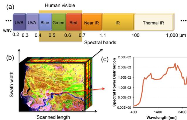
**Fig. 1:** Schematic overview of hyperspectral imaging. (a) a spectral range of wavelengths around the visible spectrum, (b) an example of a hyperspectral image, (c) an example of a measured spectrum
