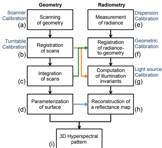
**Fig. 4:** Parallel geometric and radiometric data processing pipeline for reconstructing a hyperspectral 3D reflectance model from piecewise scans and radiance maps in the system [17].
