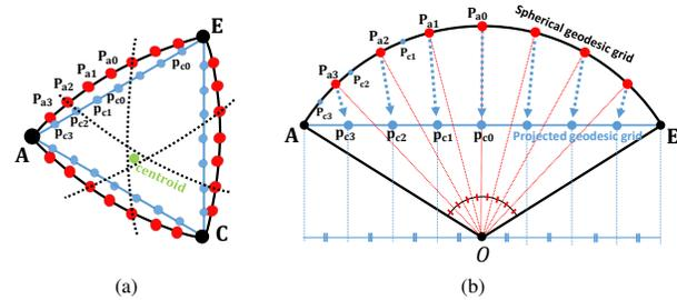
Figure 1. (a) Equal-arc subdivision on the spherical PPT. Three great arcs that are parallel to the edges of the PPT do not meet in a point. A centroid point of the triangle is defined as a vertex of the geodesic grid. (b) The transformation method of the geodesic grid using equal-arc subdivision. There is no formulated relationship but a projection algorithm using a neighboring relative position of pixels on each grid plane.
