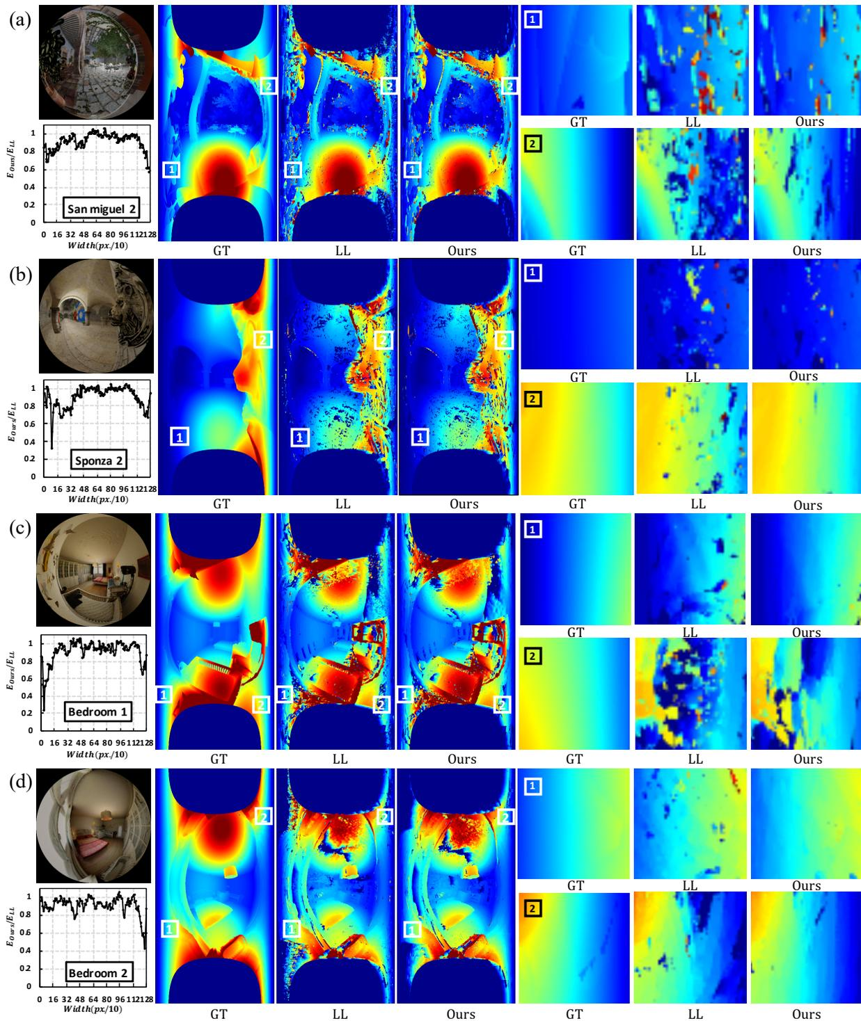
Figure 2. Results of four synthetic datasets. Left-top is the left image of fisheye stereo; left-bottom is the ratio of error pixels by 10-pixel-step in x-axis; GT disparity map; LL-based disparity map; Our disparity map; Comparison of disparity results at two identical positions.
