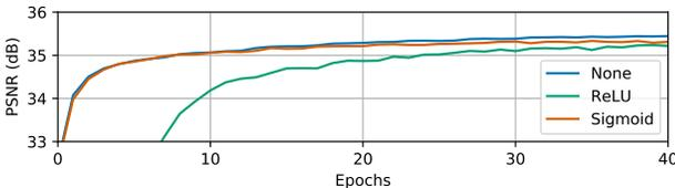
Figure 7: Impact of the activation function in the last convolutional layer in the luminance network.
