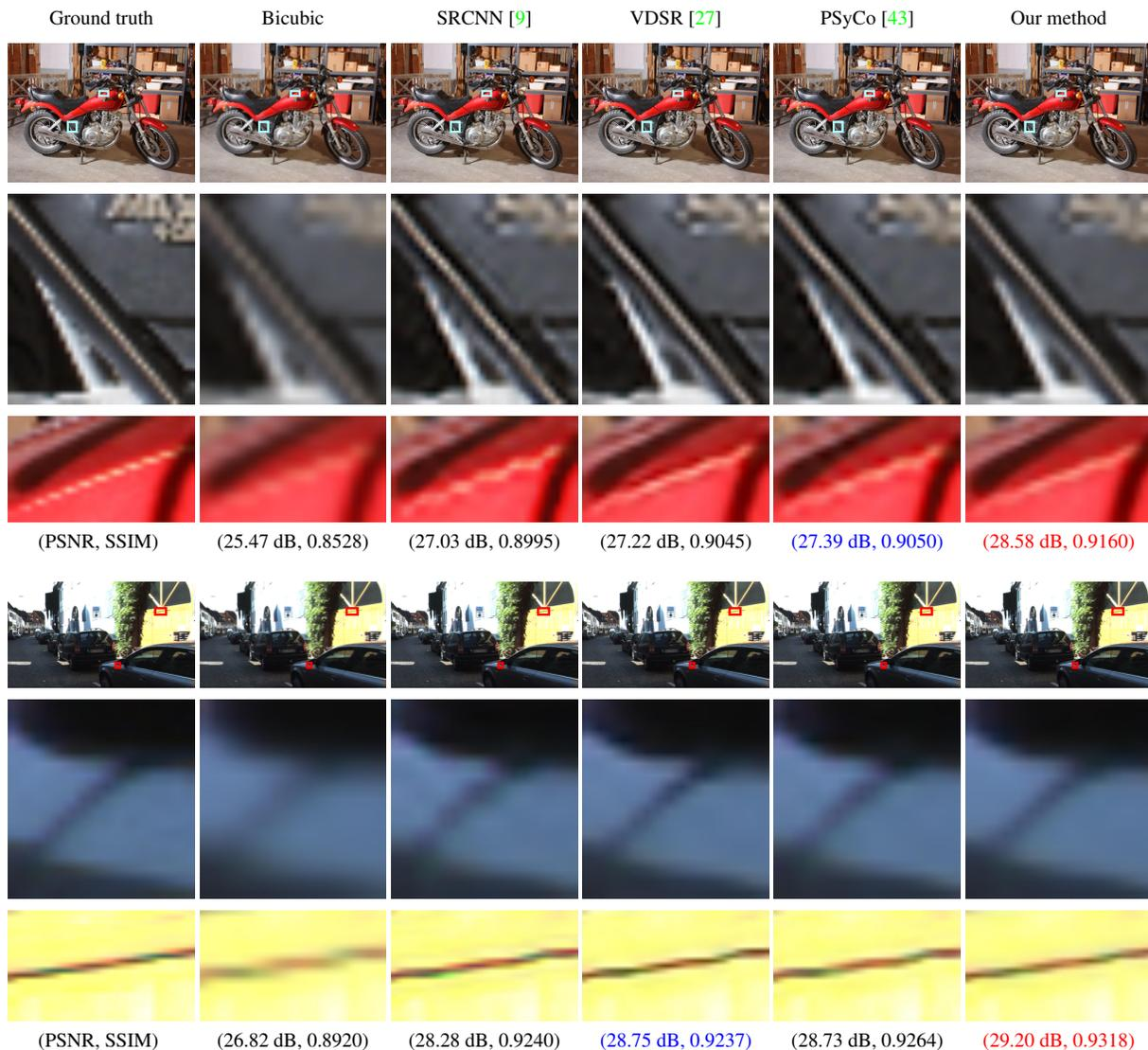
Figure 9: Results of super-resolution with the ×2 magnification factor. PSNR and SSIM values are shown under each result. The red color indicates the highest PSNR and SSIM values, and the blue color represents the second highest values.
