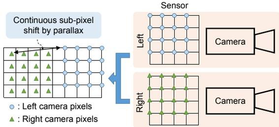
Figure 2: Registering stereo images with parallax. Affine transformation that aligns two images contains *subpixel shifts*, due to the geometric difference between perspective projection and affinity of the stereo planes. We learn a mapping from subpixel shifts to a high-resolution image.
